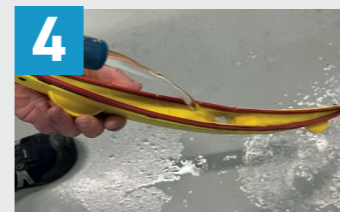
4 Remove squeegee assembly, clean by flushing water and wiping with clean cloth.
