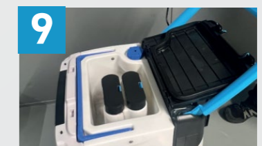
9 Leave tank cover open so it can dry naturally.
