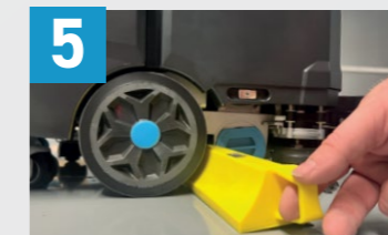
5 Remove and clean hopper.
